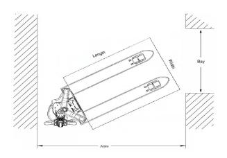
Aisle dimensions listed above assume 4" between loads. Use the larger dimension; load width or load length. For ease of use and add 6" to 12" for operator clearance to the appropriate specifications listed above. Truck performance may vary due to application requirements' and changes in model design.
