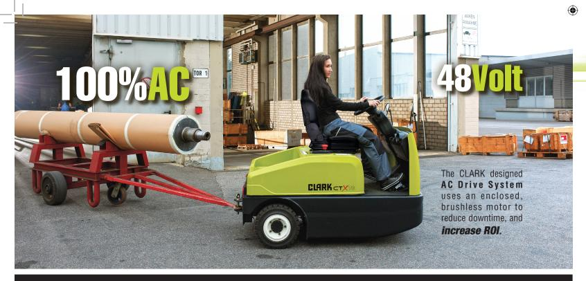
The **100% AC** 48-Volt high performance drive system, and regenerative braking, give the compact rear-wheel drive CTX exceptional acceleration, speed, and gradeability.
