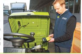
The CLARK handset can be used for diagnostics and settings of up to 20 different performance parameters to match vour requirements.
