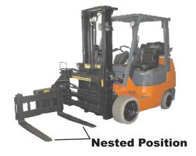
\*\*Pivoting and Side Shifting to load and unload a trailer or to retrieve a load at floor level is fine, but above the floor level, pivoting is not allowed and side shifting is only allowed in storage racks. These rules are in accordance with ANSI B56.1.
