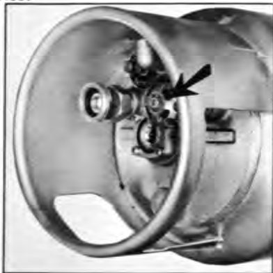
L.P. GAS SHUT-OFF VALVE
