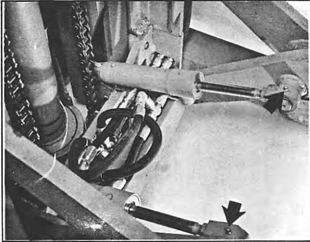
Plate 9445. Typical Pantograph Piston Rod Mounting Point Lubrication
