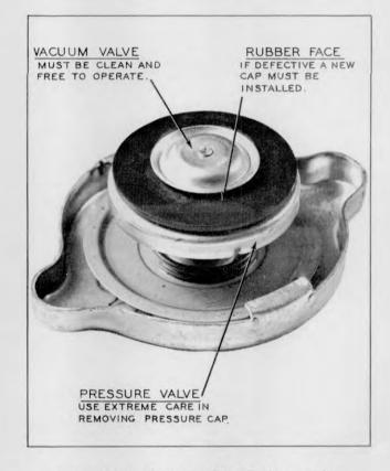
Plate 6459. Pressure Cap Gasket, Valve and Valve Gasket
