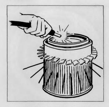
Plate 7173. Cleaning Dusty Element ELEMENT. DIRECT AIR THROUGH ELEMENT (OPPOSITE TO DIRECTION OF ARROWS CAST ON END OF ELEMENT). DO NOT DAMAGE FINS OR SEALING SURFACES OR RUP-TURE ELEMENT NOR ALLOW DUST TO DEPOSIT ON CLEAN AIR SIDE.
