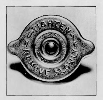
Plate 6458. Radiator Pressure Cap W A R N I N G
