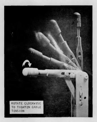
Plate 6505. Hand Brake (Actuating) Lever
