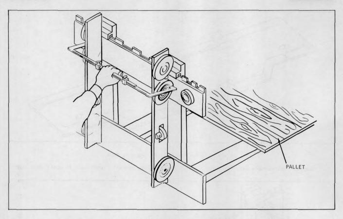
Plate 9570 Spanning Upper Rollers (Six Roller Carriage)
