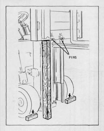
Plate 9593 Carriage Pin Replacement
