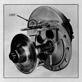
Plate 7550. Typical Axle Adapter Vent
