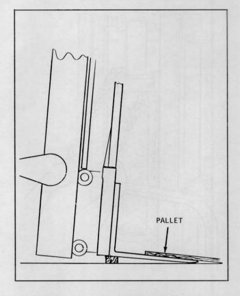
Plate 9565 Inner Rail Clearing Carriage Rollers
