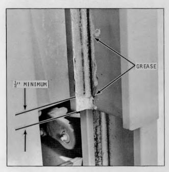
Plate 8622. Lift Chain Adjustment
