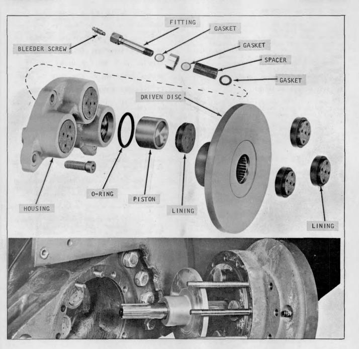
Plate 7567. Typical Service Wheel Brake Assembly
