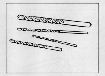
Plate 9683. Typical Twist Drills - Sizes 13/32", 3/8", 5/32", 1/8", 3/32", 1/4".
