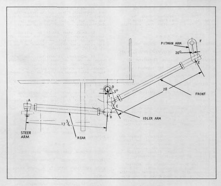
Plate 7569. Typical Steering Linkage (Side View)
