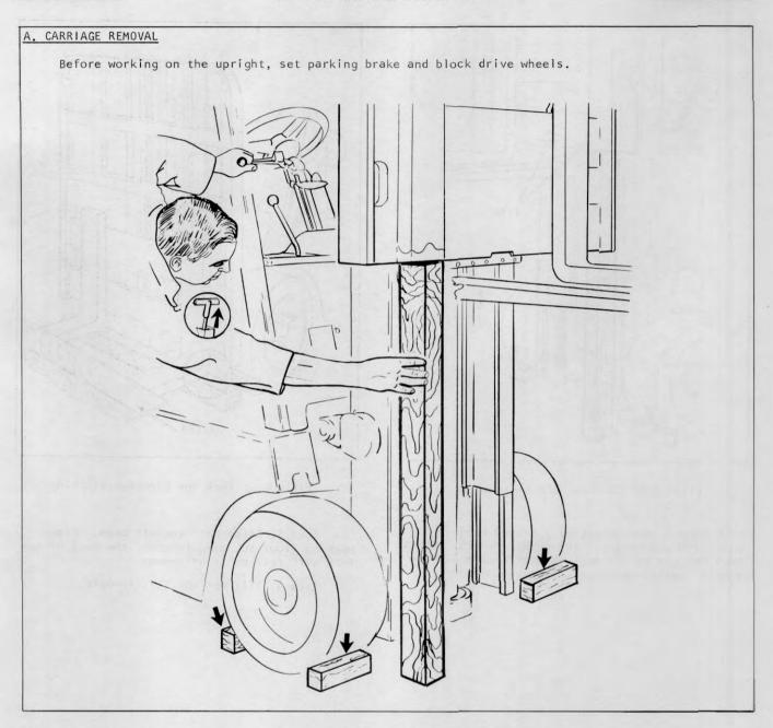
Plate 9559 Blocking Machine and Carriage
