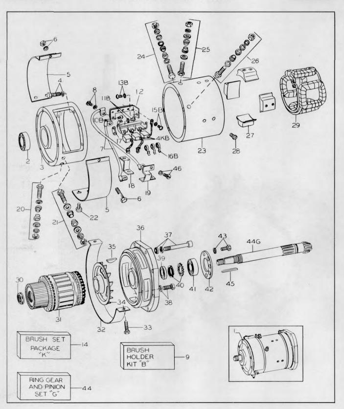
Plate 7565. Typical Drive Motor (Disassembled View)
