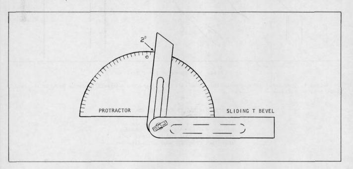
Plate 9590 Checking Roller Angle
