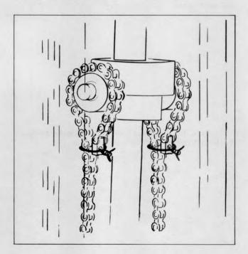
Plate 9563 Securing Chains (Typical)
