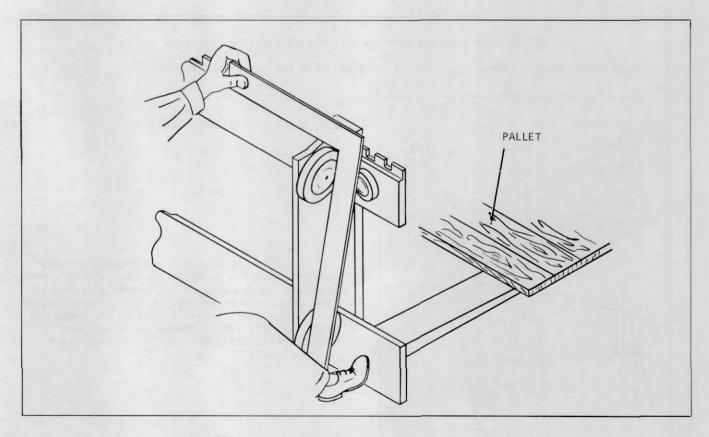
Plate 9573 Squaring Carriage Rollers (Four Roller Carriage)
