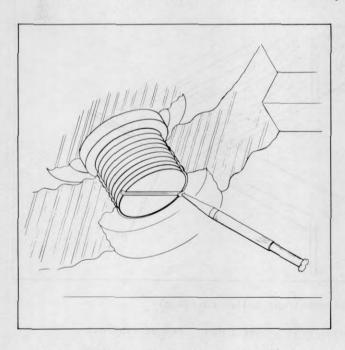
Plate 9571 Securing Outer Thrust Roller
