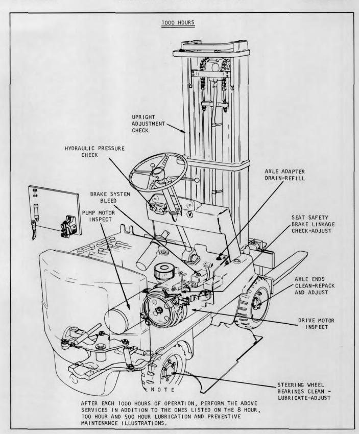
Plate \_\_\_\_\_ Lubrication and Preventive Maintenance Illustration
