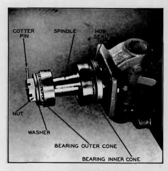
Plate 6703. Typical Wheel Bearings
