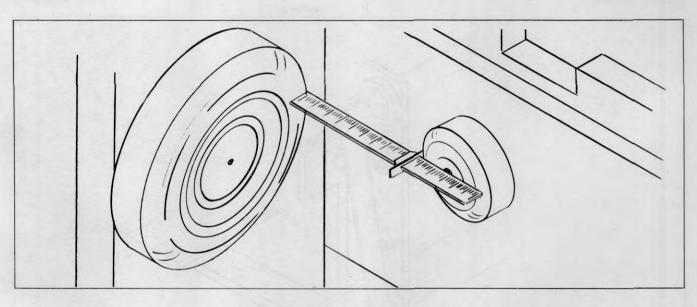
Plate 9572 Centering Carriage Rollers
