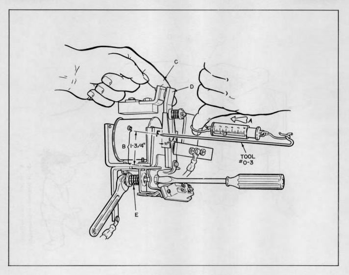
Plate 9698. Typical Armature Adjustment
