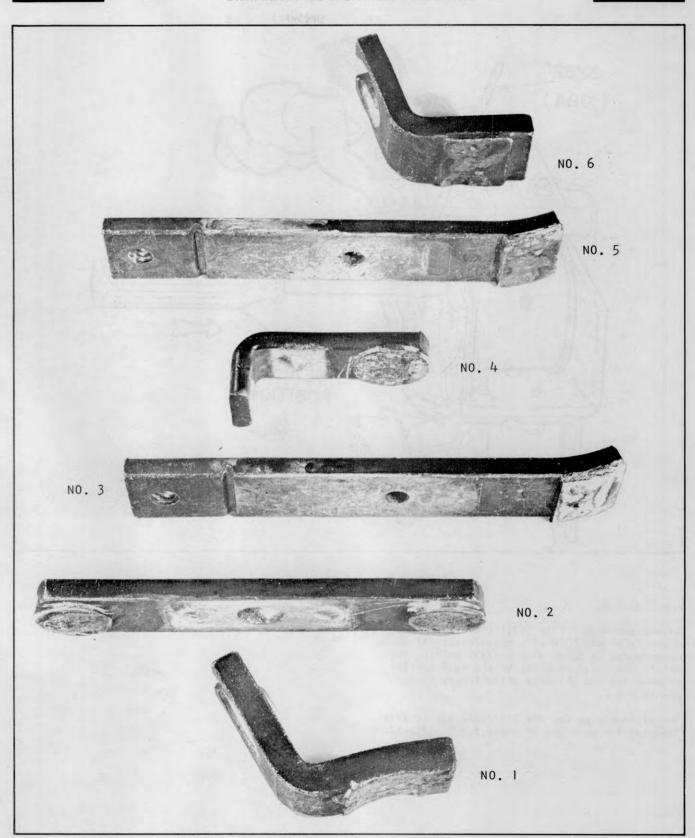
Plate 3197. Typical Contactor Tips
