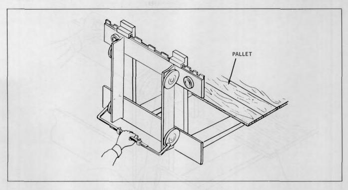
Plate 9576 Spanning Lower Rollers (Four Roller Carriage)
