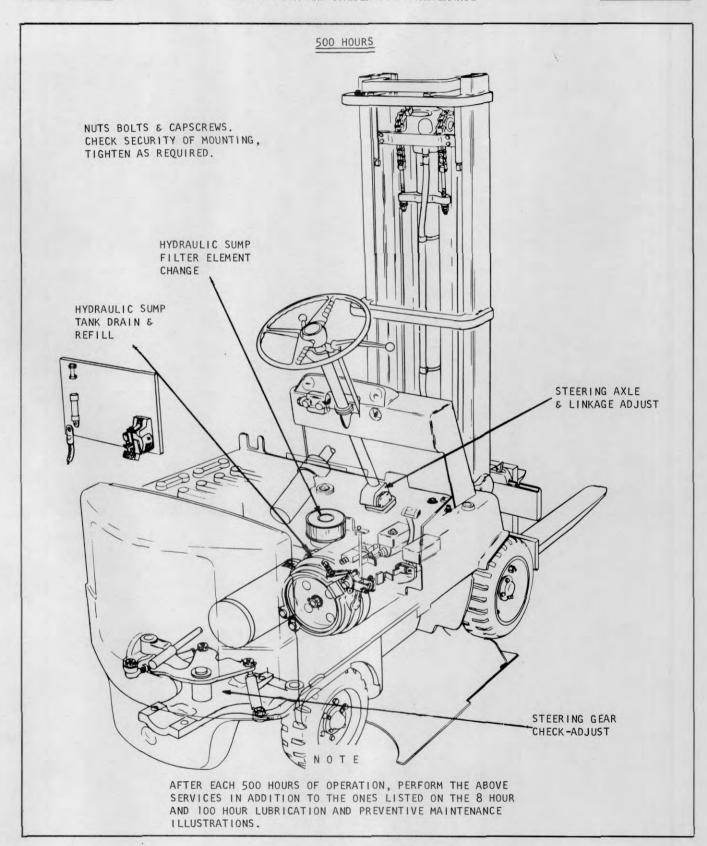
Plate \_\_\_\_ Lubrication and Preventive Maintenance Illustration
