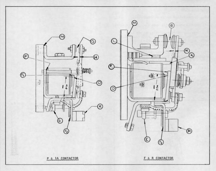
Plate 9703. Typical Contactors
