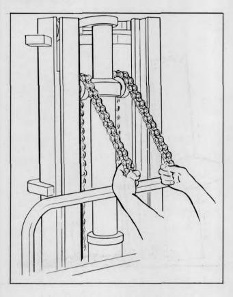
Plate 9586 Pulling Piston Head Down
