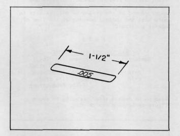
Plate 9685. Typical Brass or Steel Shim Stock .005" Thick.
