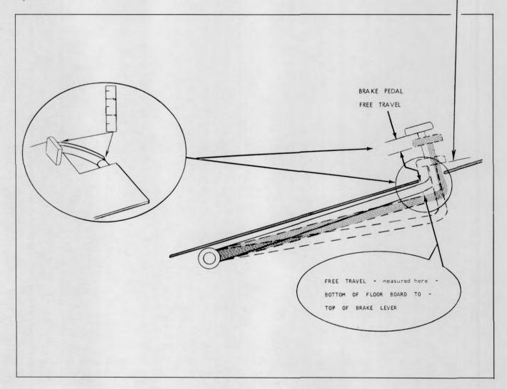
Plate 7042. Brake Pedal Check and Adjustment
