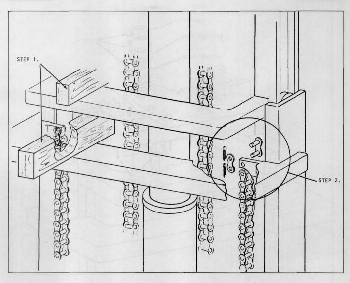
Plate 9650 Rear Lift Cylinder Removal
