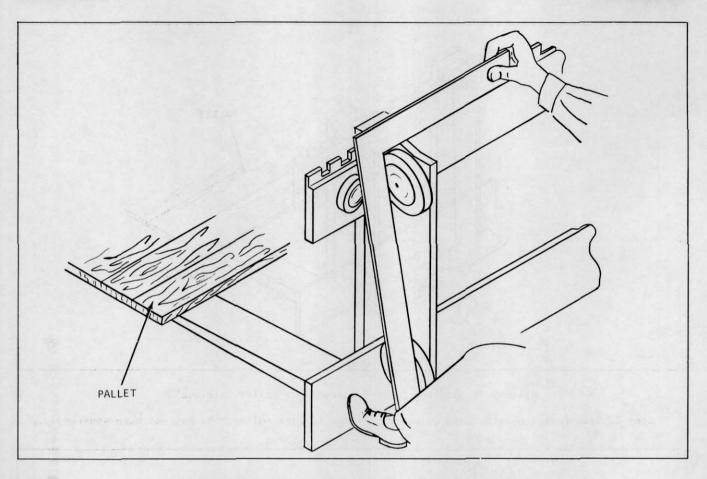
Plate 9578 Checking Squareness (Four Roller Carriage)
