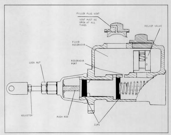
Plate 7339. Brake Pedal Adjustment
