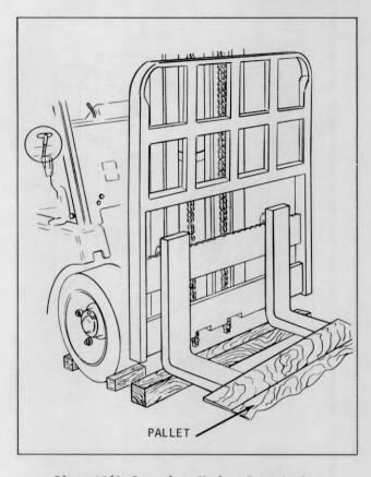
Plate 9562 Removing Chains From Anchors
