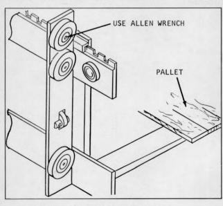
Plate 9581 Removing Top Roller
