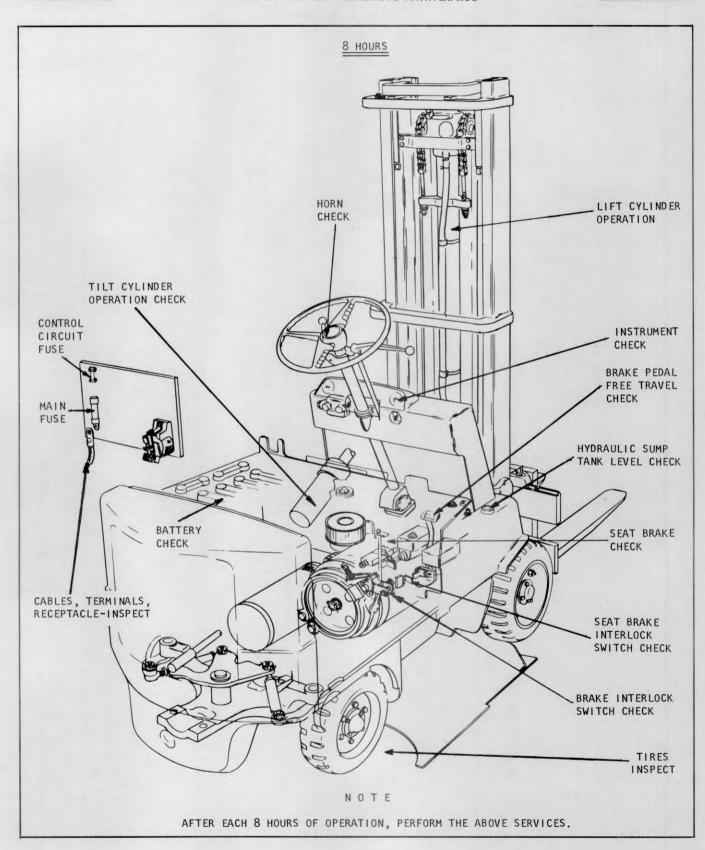
Plate \_\_\_\_ Lubrication and Preventive Maintenance Illustration
