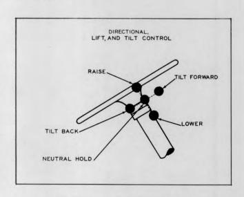
Plate 4448. Hydraulic Control Lever
