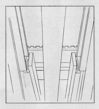
Plate 9591 Rollers Guiding Into Inner Rail
