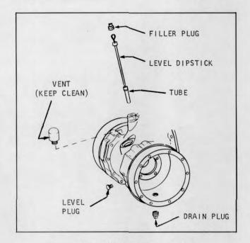
Plate 7549. Typical Axle Adapter
