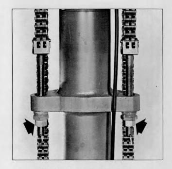
Plate 6634. Lift Chain Adjustment (Chain Anchor Rods)
