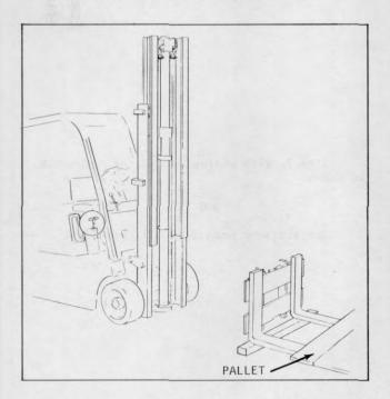
Plate 9566 Backing Machine Away From Carriage
