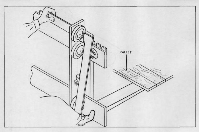
Plate 9574 Square And Side Thrust Roller
