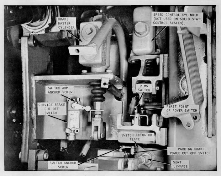
Plate 7545. Parking Brake (Deadman) Power Cut Off Switch; check Service Brake (Interlock) Power Cut
