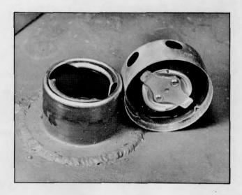
Plate 7046. Typical Hydraulic Sump Tank and Sump Breather
