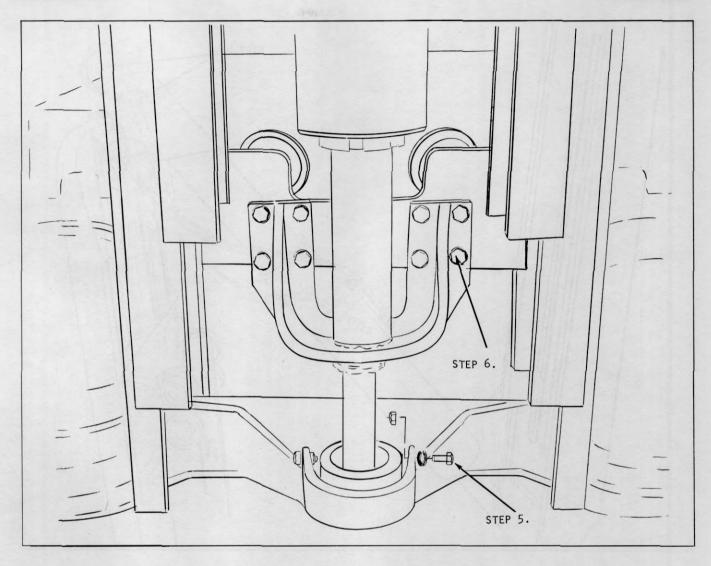
Plate 9652 Cylinder Lifting Bracket
