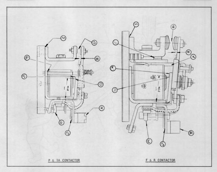
Plate 9703. Typical Contactors
