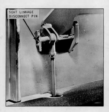
Plate 7410. Seat Linkage Disconnect Pin
