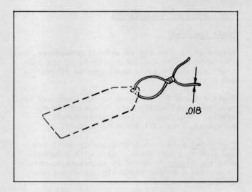
Plate 9682. Typical Tag Wire .018 Diameter Maximum.
