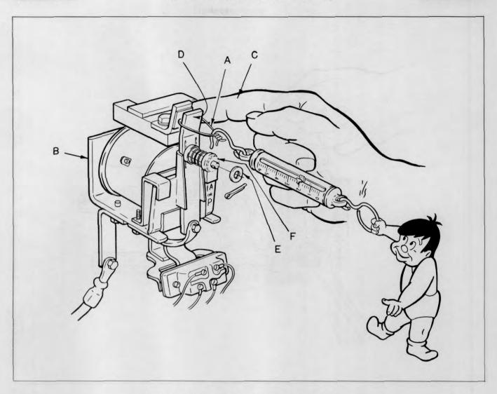
Plate 9697. Typical Spring Adjustments
