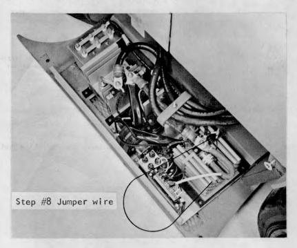
WITH DRIVE WHEELS JACKED UP AND INSULATOR IN POWER TIP GAPS OF 1A AND FW CONTACTORS, CHECK MAXIMUM SPEED VOLTAGE AND CURRENT LIMIT. THESE ADJUSTMENTS HAVE BEEN PRESET AT THE FACTORY AND SHOULD NOT REQUIRE ADJUSTMENT.
