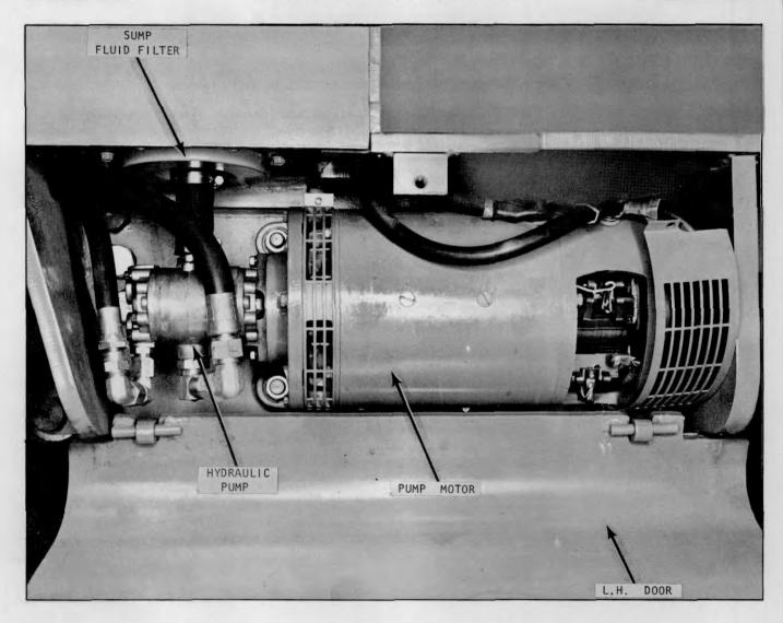
Plate 7556. Sump Tank, Filter and Pump
