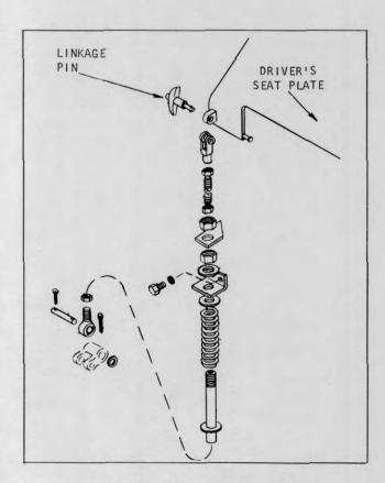
Plate 7548. Parking Brake Linkage
