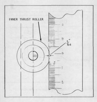
Plate 9585 Reading Roller Projection
