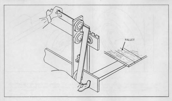
Plate 9574 Squaring Carriage Rollers (Six Roller Carriage)
