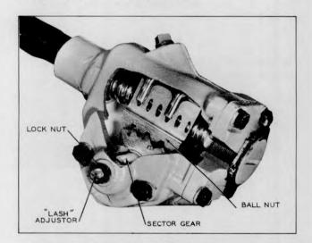
Plate 6637. Steering Gear Lash Adjustment (Sector Gear)
