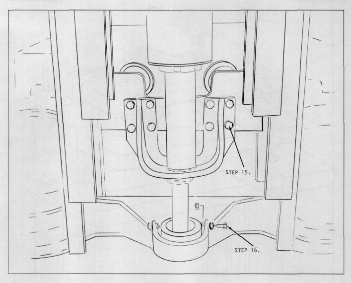
Plate 9658 Cylinder Lift Bracket
