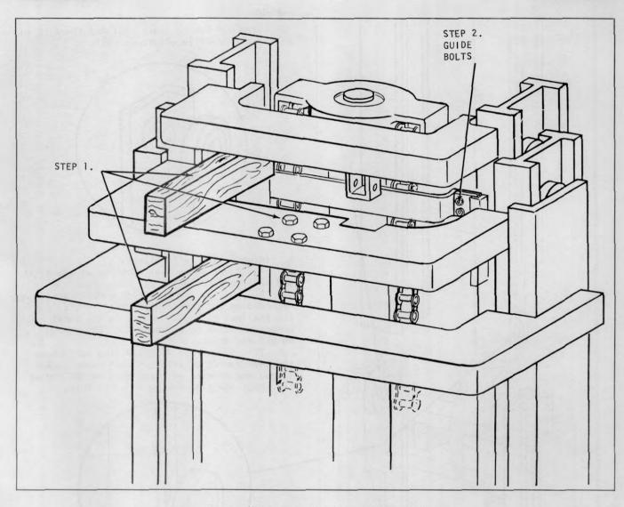
Plate 9642 Standard Triple Piston Head
