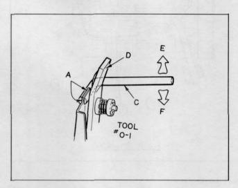
Plate 9692. Typical Wipe Adjustment
