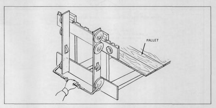
Plate 9577 Spanning Lower Rollers (Six Roller Carriage)
