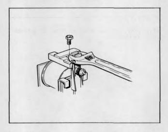
Plate 9690. Typical Contactor Arm Alignment
