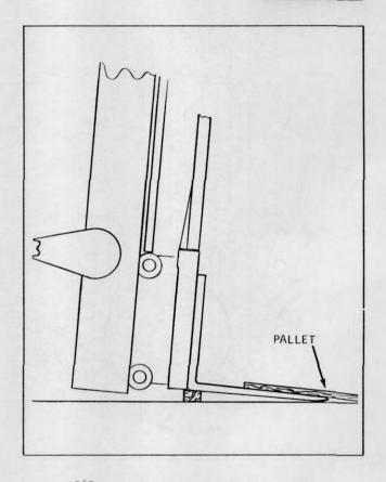
Plate 9565 Inner Rail Clearing Carriage Rollers
