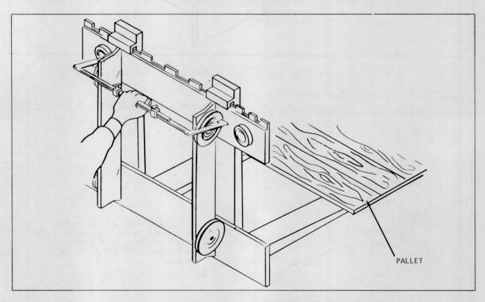
Plate 9569 Spanning Upper Rollers (Four Roller Carriage)
