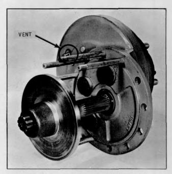
Plate 7550. Typical Axle Adaptor Vent
