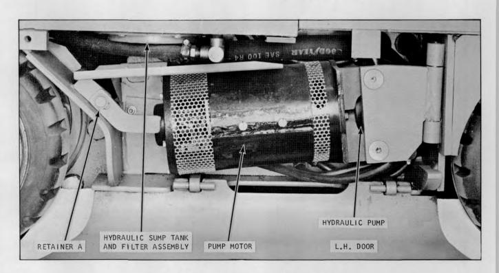
Plate 8661. Sump Tank, Filter and Pump
