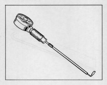
Plate 9680. Typical Spring Tension Gage.... Clark Part # 886717.
