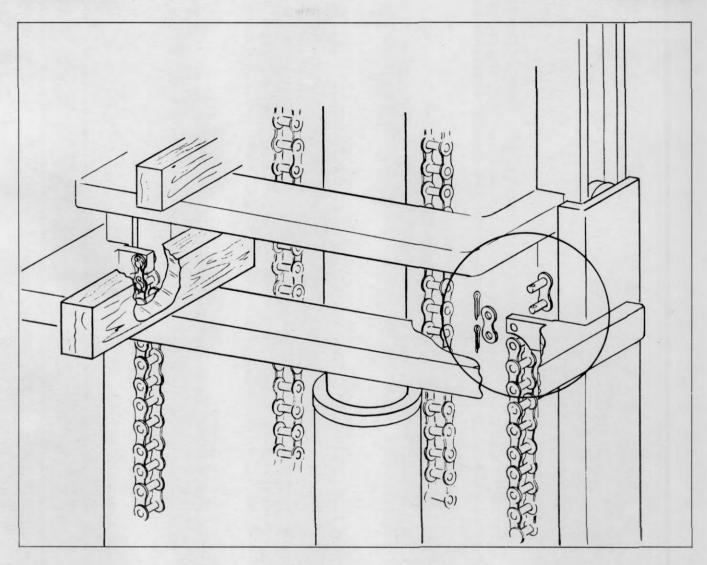
Plate 9660 Replacing Rear Lift Chains
