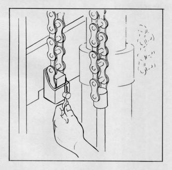
Plate 9588 Installing Cotter Pins
