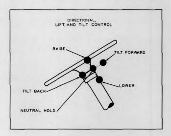
Plate 4448. Lift and Tilt Lever
