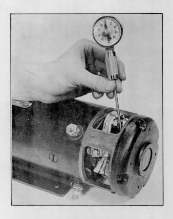
Plate 6560. Typical Method Checking Brush Spring Tension
