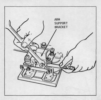
Plate 9694. Typical Gap Adjustment
