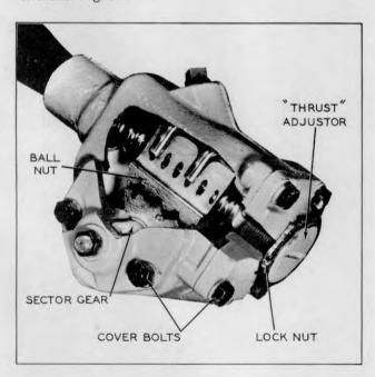
Plate 6636. Steering Gear Thrust Adjustment (Worm Bearings)
