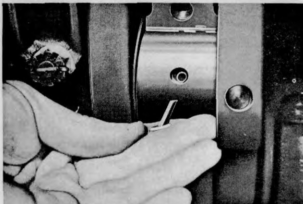
Figure 46 — Removing Main Bearing
