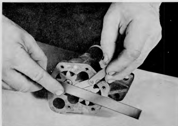
Figure 69 — Checking Oil Pump End Clearance
