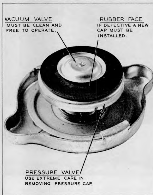
Plate 6459. Pressure Cap Gasket, Valve and Valve Gasket
