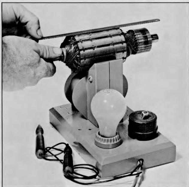
Plate 6996. Checking Armature For Short Circuit
