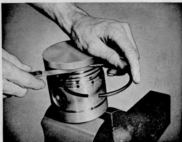
Figure 41 — Checking Ring Clearance in Groove
