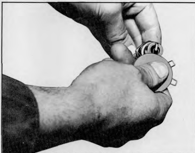
Plate 3278. Check Spark Plug Gap
