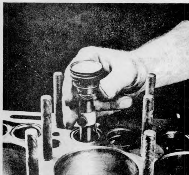
Figure 23 — Indicating Valve Seat
