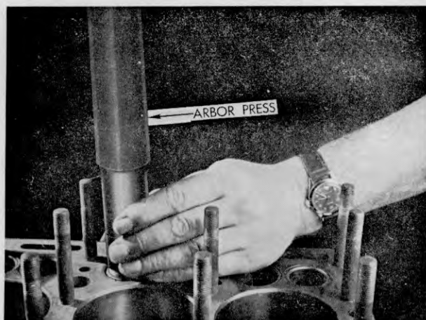
Figure 21 — Installing valve seat insert with an arbor press
