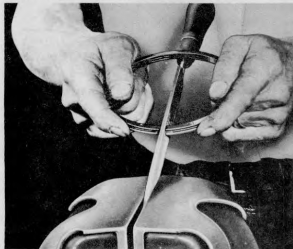
Figure 41 — Filing piston ring to increase gap
