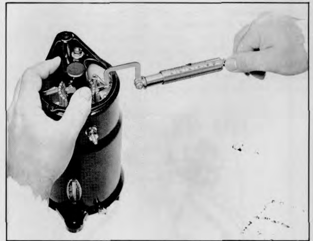
Figure 1. Measuring Brush Spring Tension
