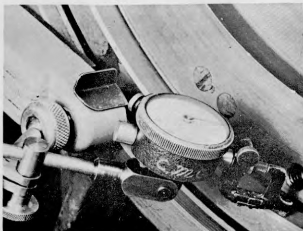
Figure 73 — Checking Flywheel Counterbore
