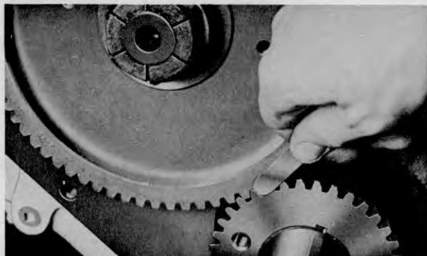
Figure 55 — Checking Timing Gear Backlash Gears marked same as the original as far as sizes are concerned should be used as replacements.
