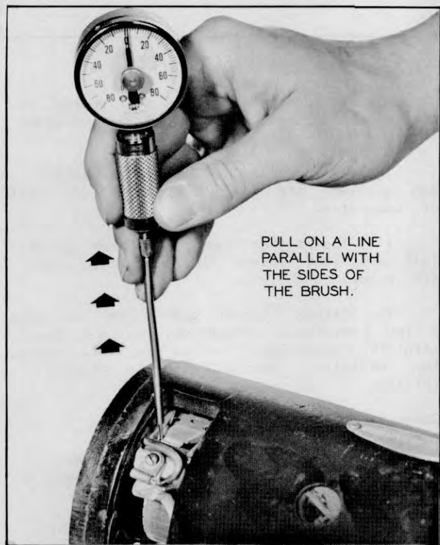
Plate 6450. Checking Brush Spring Tension
