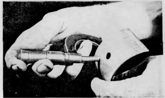
Figure 47 — Measuring Bearing Thickness
