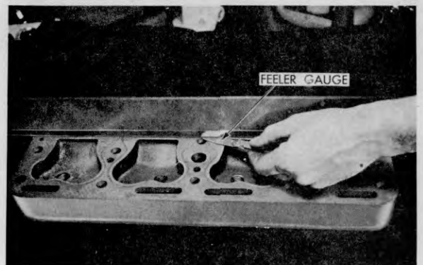
Figure 13 — Checking cylinder head flatness lengthwise.
