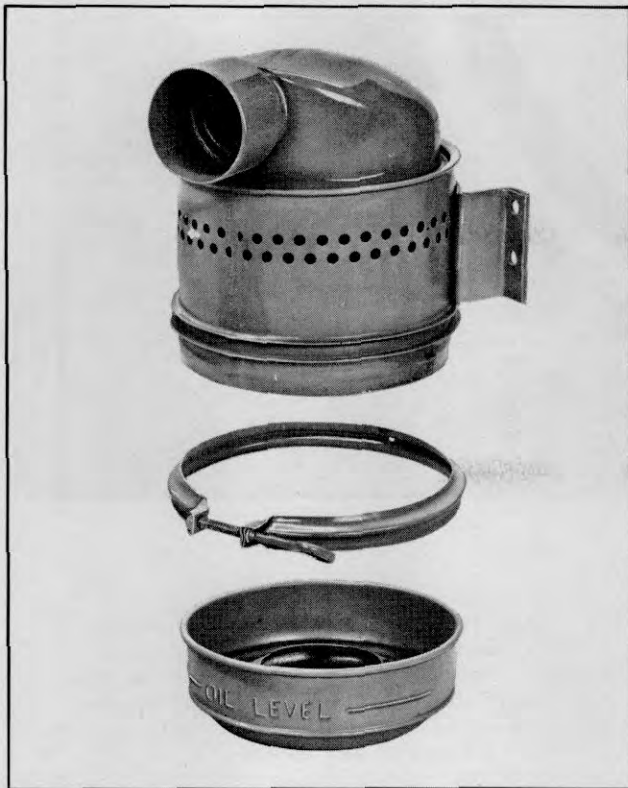
Plate 5985. Air Cleaner Fill to oil level only.
