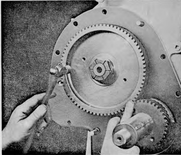
Figure 59 — Checking Gear Fit
