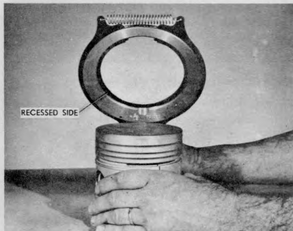
Figure 42 — Installing Rings with Ring Expander Tool
