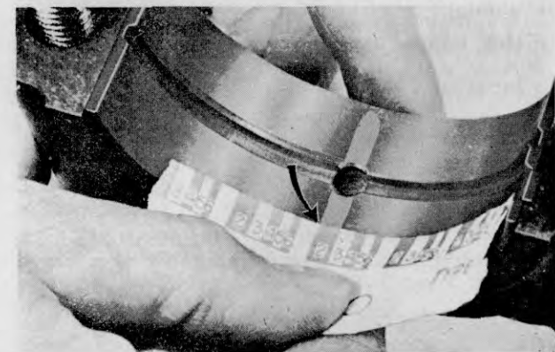
Figure 48 — Checking Bearing Clearance with Plastigauge
