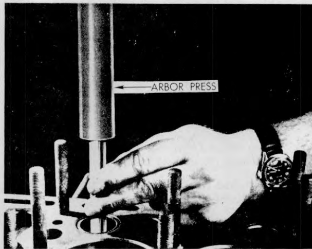
Figure 18 — Removing valve guides
