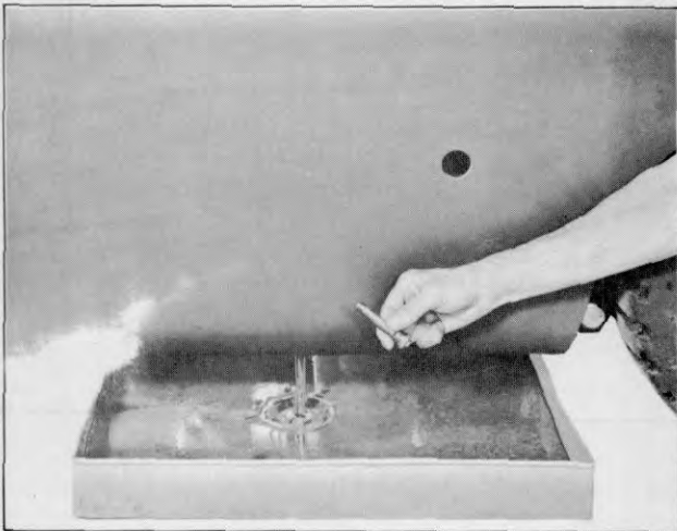
Plate 5359. Draining Sump Tank
