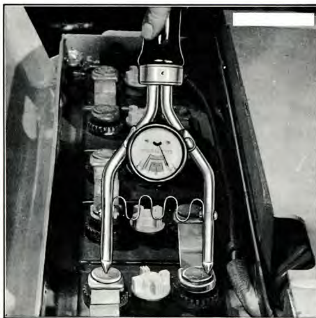
Plate 4008. Charge Test Fork Check
