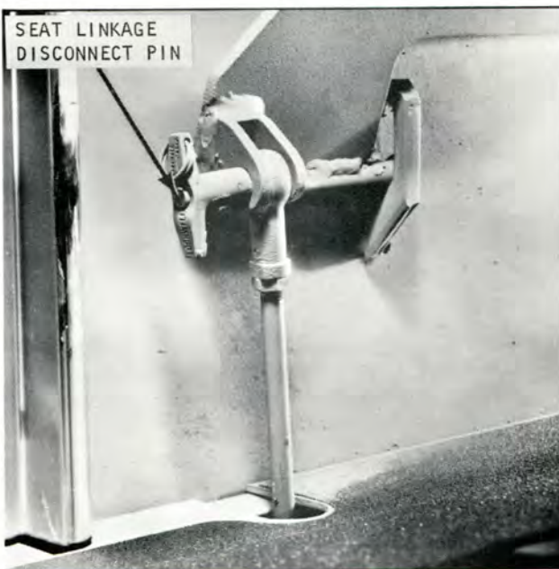
Plate 7410. Seat Linkage Disconnect Pin
