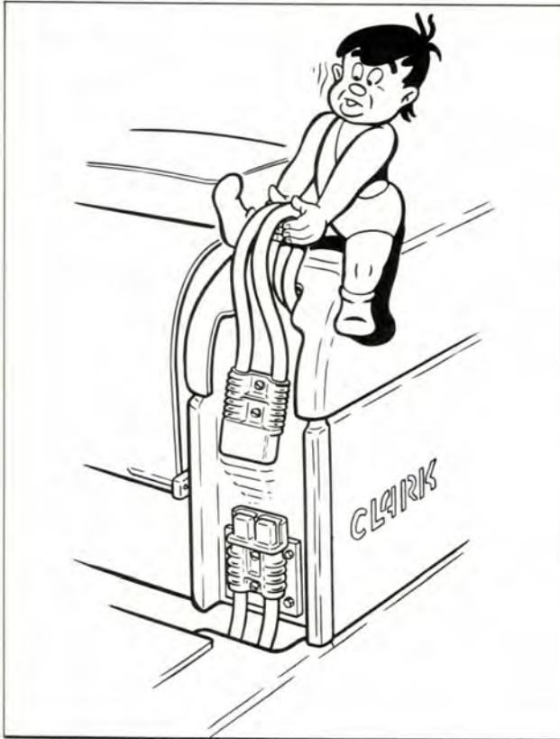
Plate 9688. "Typical" Battery Disconnect
