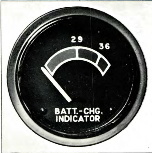
Plate 7388. Battery Charge Indicator
