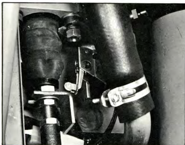
Plate 7615. Brake Interlock Switch
