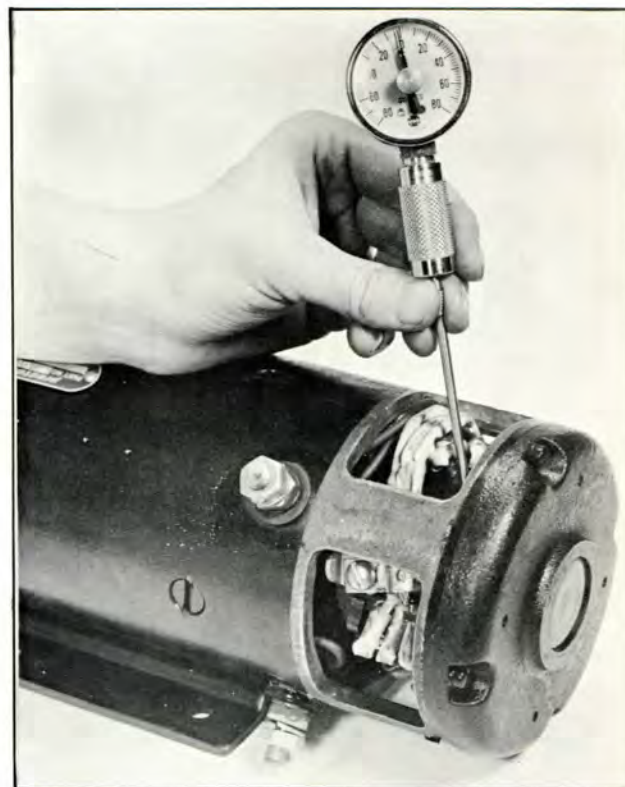
Plate 6560. Typical Method Checking Brush Spring Tension
