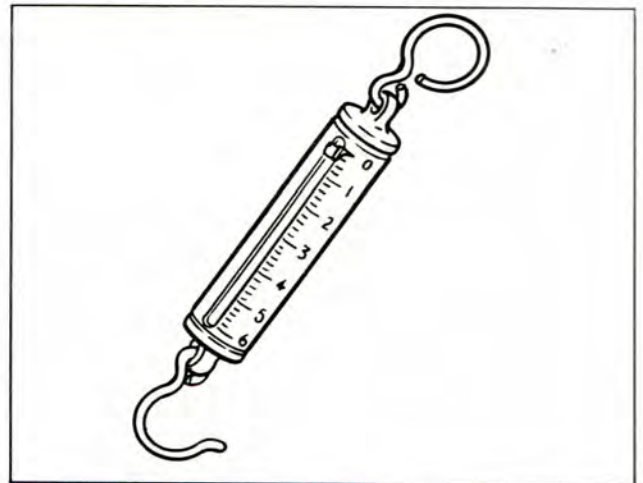
Plate 9679. Typical Instrument Type "T" - Chatillon Spring Tension Gage, Mfg. by Chatillon Inst. Co., New York, N.Y.
