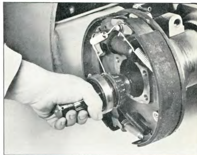
Plate 7479. Removing Axle Shaft
