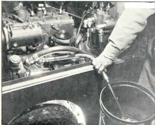
Plate 3720. Removing Hydraulic Sump Oil
