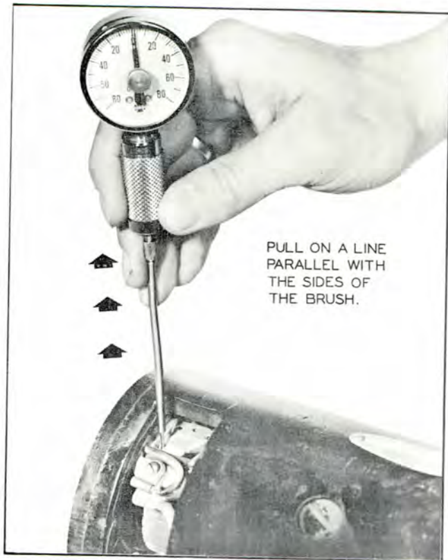
Plate 6450. Checking Brush Spring Tension
