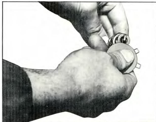
Plate 3278. Check Spark Plug Gap
